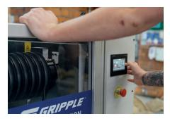
The Enhanced & XL DeReeler features one-touch reel loading and unloading, capable of handling wire reels up to 300kg in weight (with XL DeReelers handling up to 400kg), and wire diameters ranging from 0.5 to 6 millimeters.
