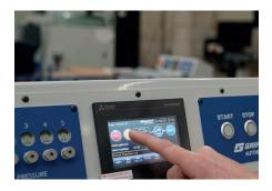
With a user-friendly HMI interface, you can easily program specific wire lengths and batch quantities for a fully automated experience. Plus, our adjustable power output allows you to dial in the correct power for your specific fuse requirements.
