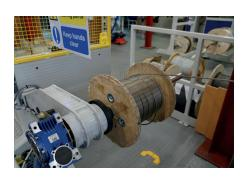
The DeReeler is capable of handling wire reels weighing up to 1000kg with diameters of up to 10 millimetres.
