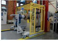
The DeReeler can process approximately 1 meter of wire per second, depending on the reel size.
